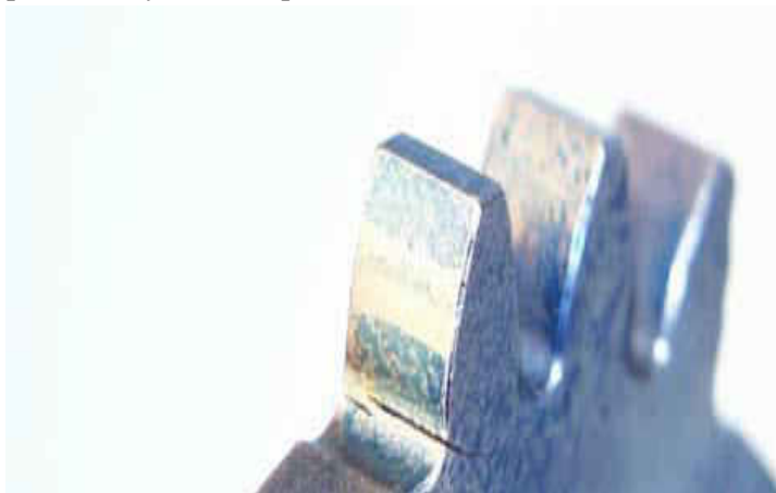
Figure 5: Single tooth bending fatigue failure at the end of test. [2]
