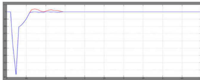
Figure 9 : Voltage at PCC and Three phase Source (a) Without Control (b) With control
