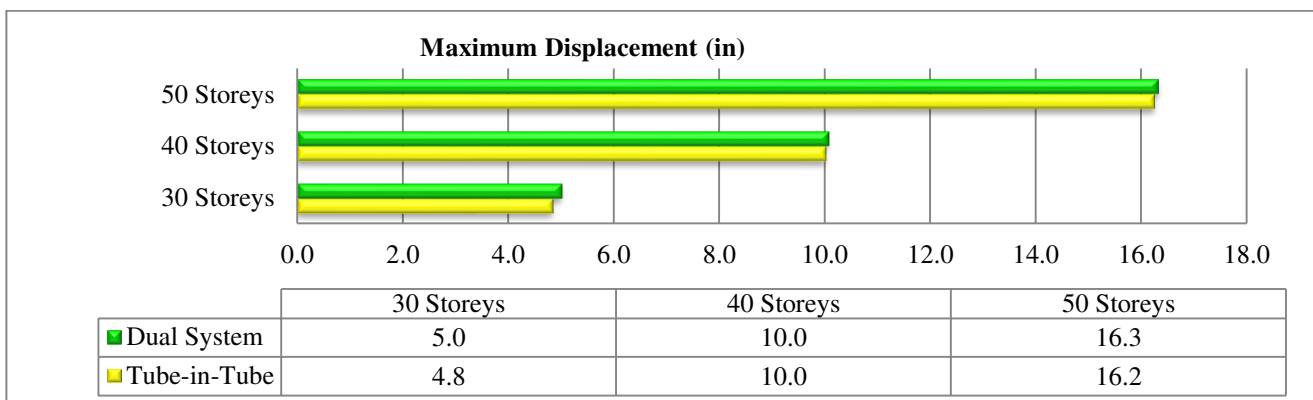
Figure 12. Comparison of Maximum Displacement between 30, 40 and 50 Storeyed Tube-in-Tube Structure Buildings and Dual System Buildings (multiplying with Modification Factor) in X direction
