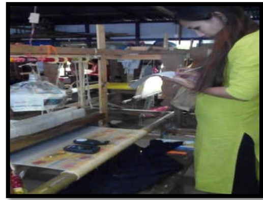
Plate 8: Reading of artificial illumination level taken on a work centre
