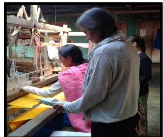
Plate 4: Reading of noise level taken on a work Centre
