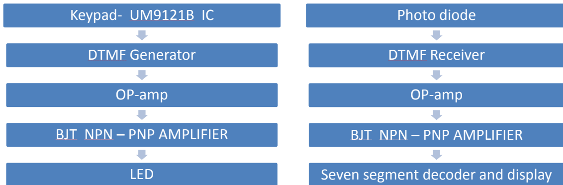
Figure 1: Flow Diagram for DTMF Transmitter (Left) and Receiver (Right)
