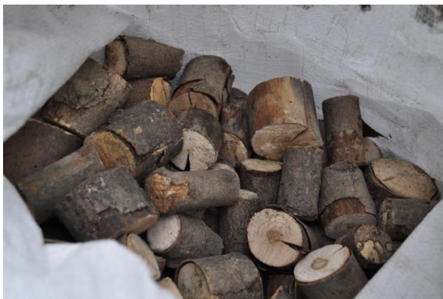
Figure 2. Wood Chunks used to power the Downdraft Gasifier [23]
