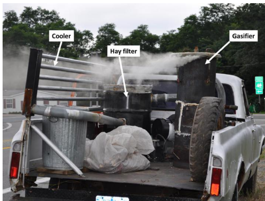
Figure 2. 1969 GMC Truck Powered by a Downdraft Gasifier [22]
