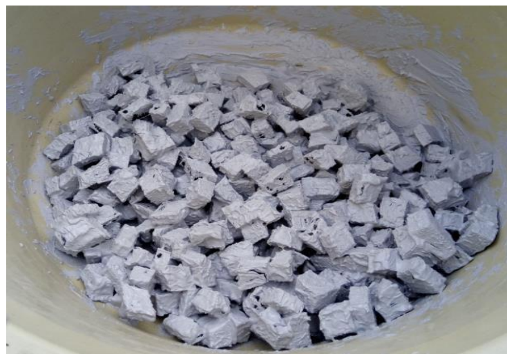
Figure 2 Waste rubber tyre particles coated epoxy resin
