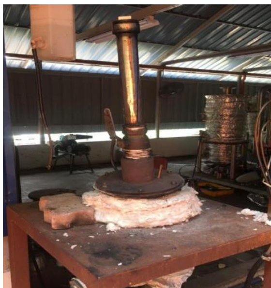
Fig. 2.2 Pyrolysis reactor for production of bio-oil
