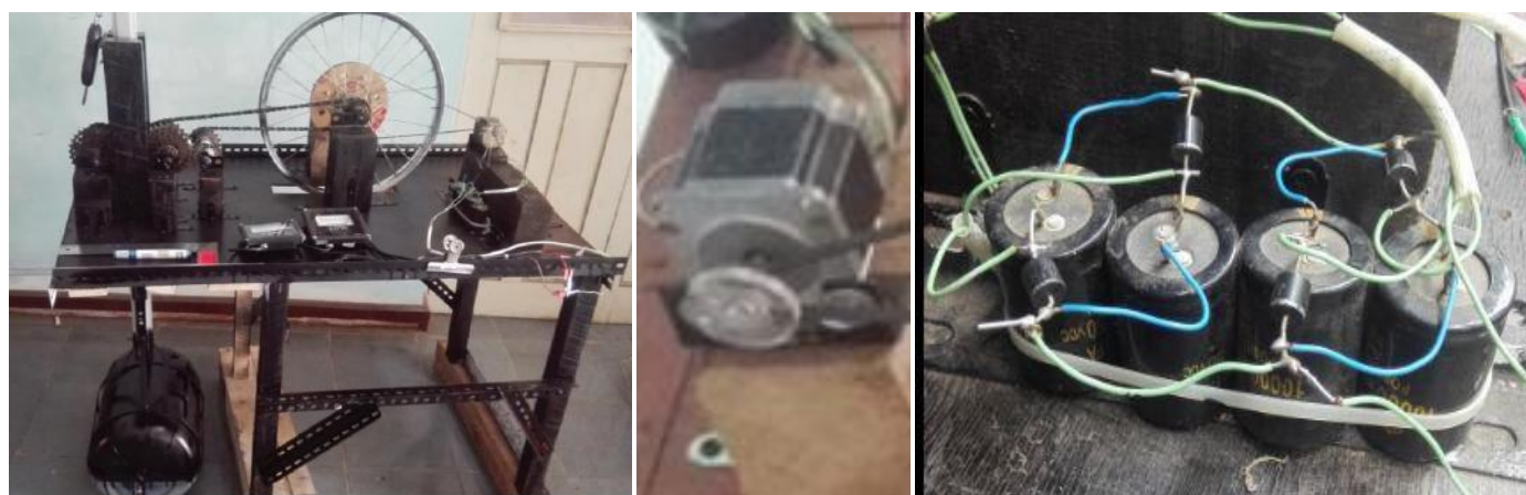
Figure 5.1. (a) Proposed (a) Wave Energy Converter, (b) Permanent Magnet Rotating Machine and (c) Voltage Doupler Rectifier
