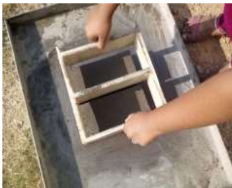
Fig.4 Demoulding of bricks
