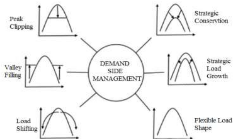
Fig.1 The six main types of load shape objective in Demand Side Management (DSM).
