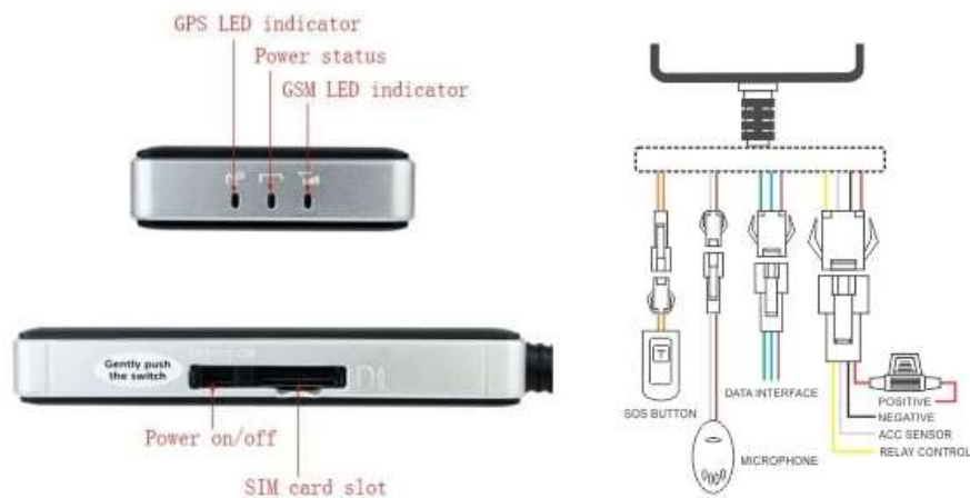
Figure 2. GT06N wiring diagram
