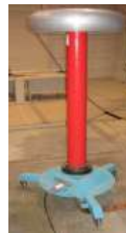
Figure 4. Resistive voltage divider of the generator TABLE 1
