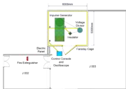
Figure 6. Layout of the Laboratory and earth connections
