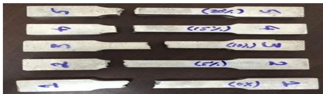
Fig 19: Piece after breaking in UTM
