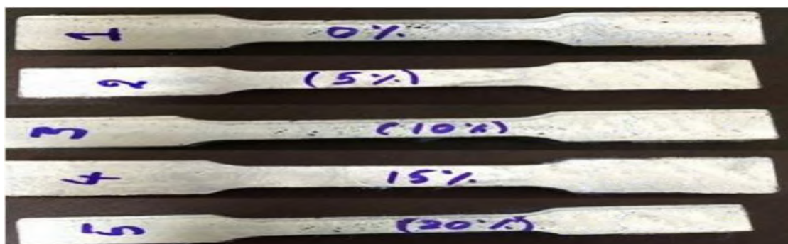
Fig 18: Piece before breaking in UTM
