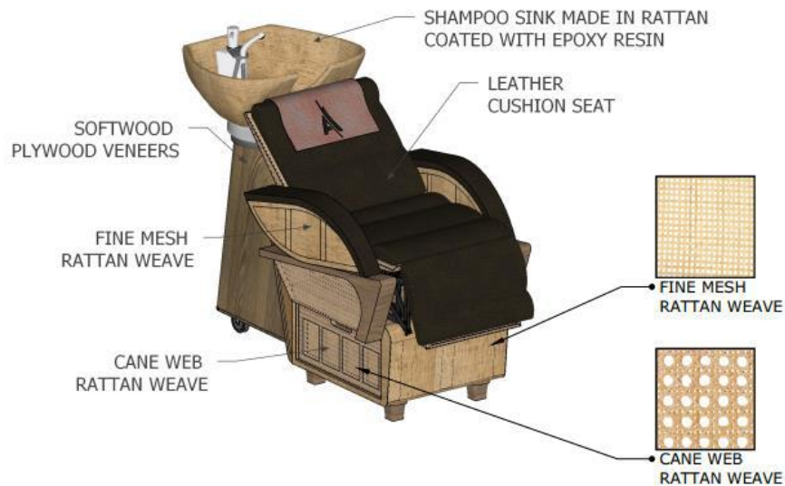
Figure 3. Major components of the rattan-based shampooing bed.
