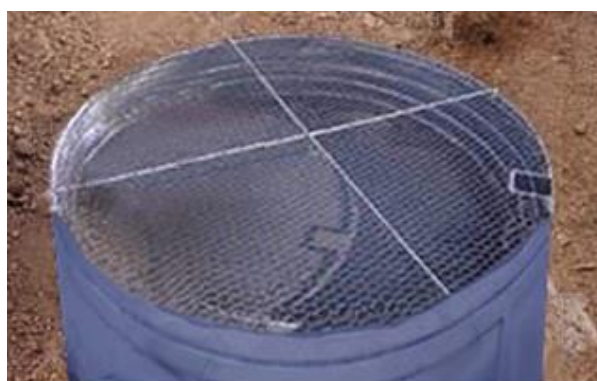
Figure 24. Construction and appearance of type "A" evaporator
