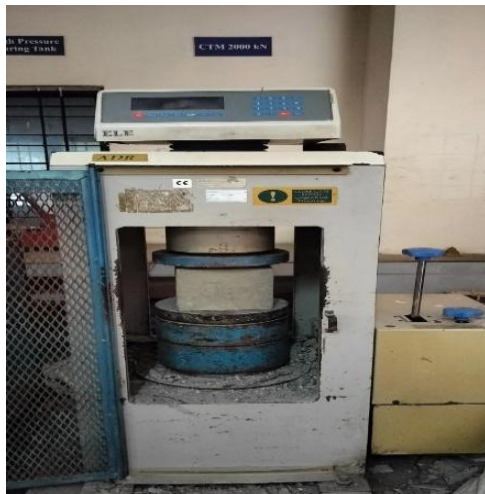
Figure 7: Testing of GPC cubes in CTM
