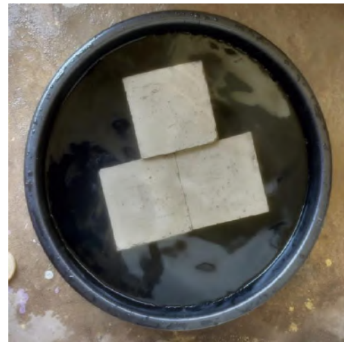
Figure 8: GPC cubes immersed in water
