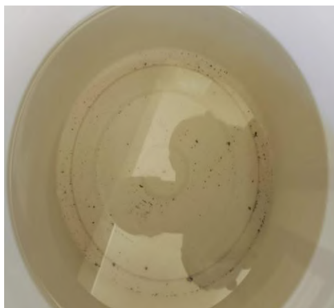
Figure 9: Change of color of water due to leaching of Sodium silicate
