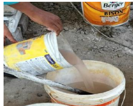
Figure 4: Mixing of NaOH & Na 2 SiO 3 solution
