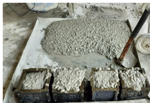
Figure 6: Casting of GPC in moulds
