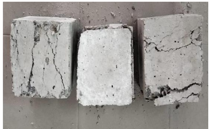
Figure 10: GPC cubes after compression test.
