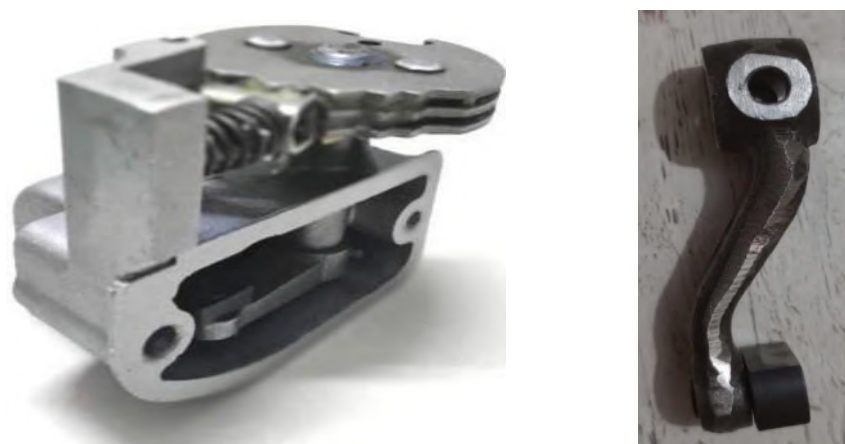
Fig. 1. The gear shifting mechanism and gear shifting fork[2]
